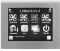
The fresh air system can be left on "auto" but you can press the boost button during cooking or if the bathroom is steamy. If you go away during the winter leave it on the lowest speed '1' to ensure warm fresh air on vour return.
