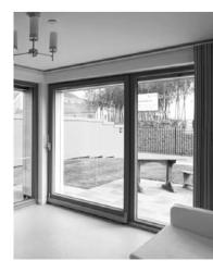
To keep cool in the summer take advantage of colder night time temperatures outside and leave the windows open in the secure "tilt" position overnight. If it's hotter outside in the day you can shut the windows and external blinds and then run the heat recovery ventilation to keep cool inside.
